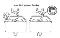
Anyone with an in-ground sprinkler or irrigation system will be required to have an approved, testable backflow prevention devices on lawn irrigation systems. They must also provide proof that the backflow prevention device has been inspected by a certified tester. Whitinsville Water Company provides this service.
